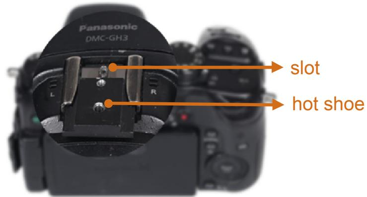
Figure 5 push the hot shoe into the slot
