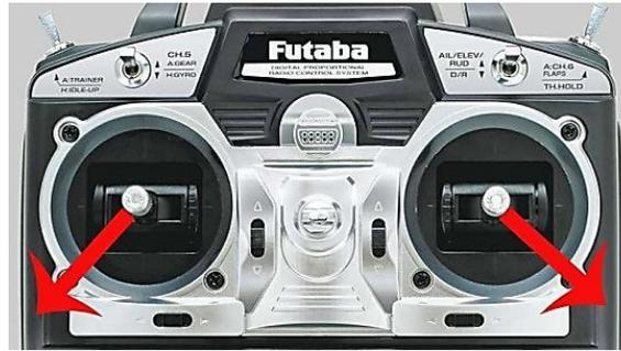
Figure 9 Resetting the gimbal Gyro ((example with Japanese Hand))
